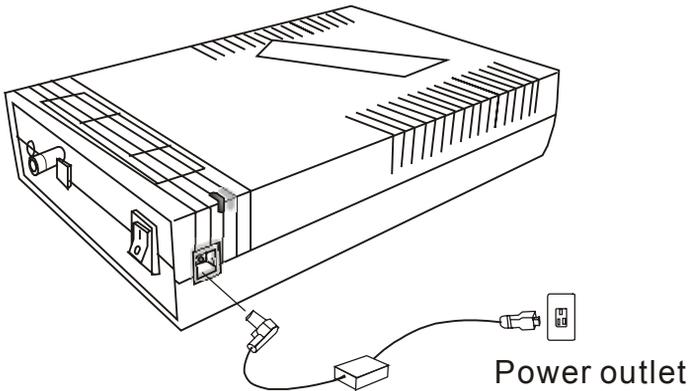
3. Turn the drive's power switch on. The drive's power indicator light should be lit.
