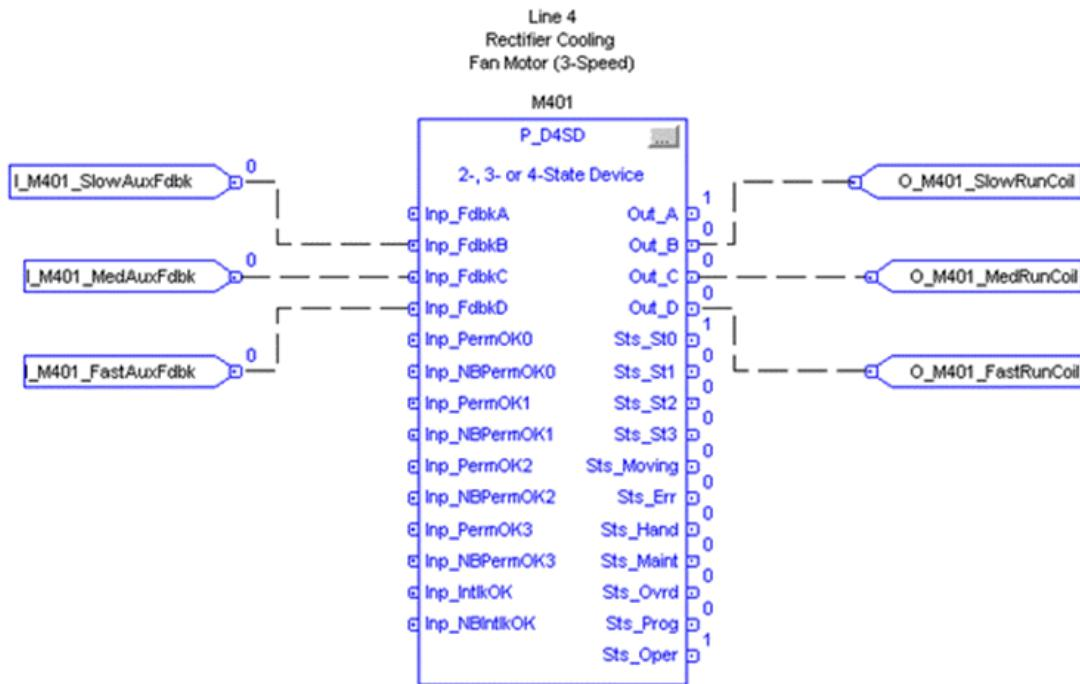
In this example, the four cooling fan states are being mapped to the device as follows:
