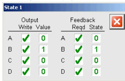
This display directs how the P\_D4SD instruction commands the device state via outputs and determines the actual device state via feedback inputs. The first two columns for output set parameters, Cfg\_OutSt[x]Write, and Cfg\_OutSt[x]Value, determine how outputs are written to command to a state. The second two columns for feedback set parameters, Cfg\_FdbkSt[x]Check, and Cfg\_FdbkSt[x]State, determine how the state is interpreted from the input values.
