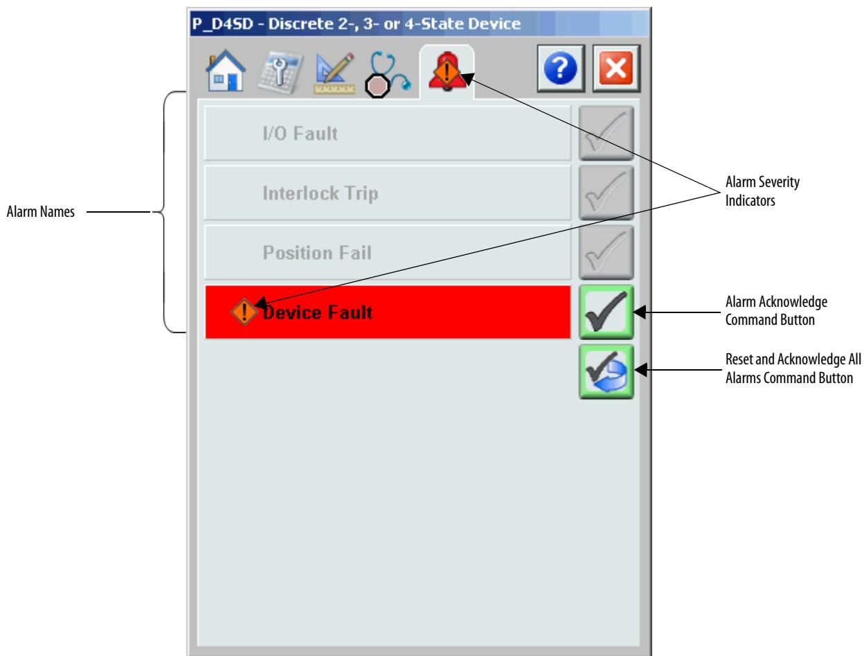
Click an alarm name to open the P\_Alarm faceplate for that alarm. From the P\_Alarm faceplate, you can configure and perform additional operations on the alarm.
