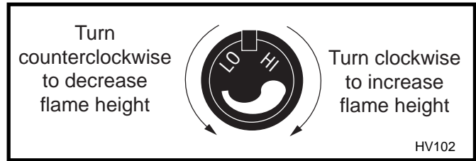
Fig. 29 Flame adjustment knob for Honeywell Valve.
