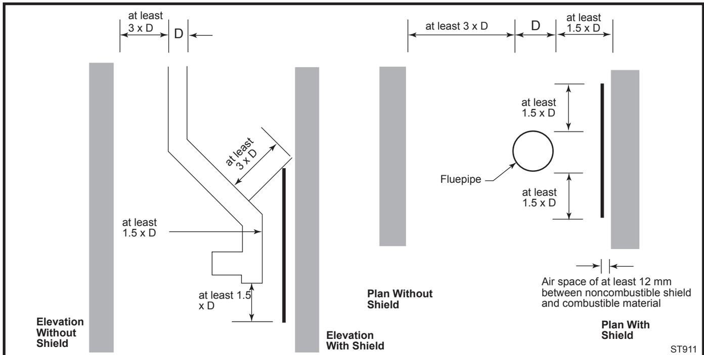
Fig. 13 Connecting fluepipe clearances.
