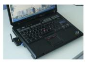
3. The LED will light after 5 to 6 seconds. If the LED does not light, it indicates that the data card is not inserted properly, or there is a malfunction with the data card or laptop.
