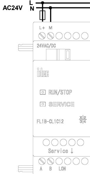
Protect the LONWORKS® Communication Module with a 80 mA/slow action fuse, if desired (recommended).
