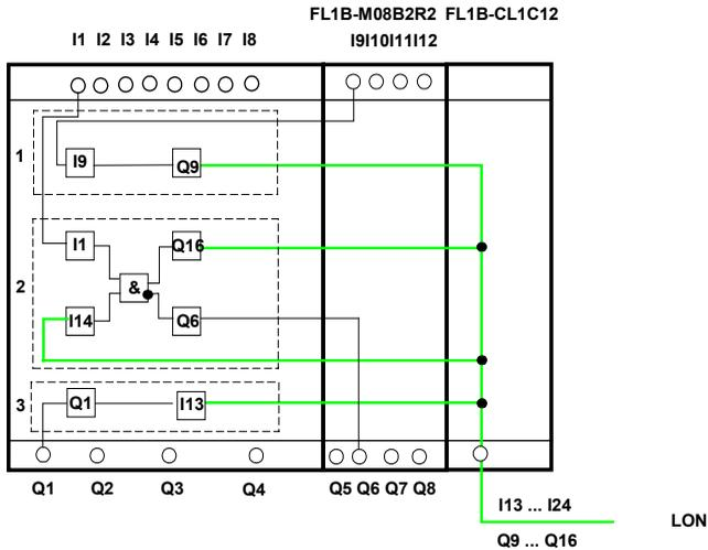
1. To map the IEC SmartRelay inputs (I1 to I8/I12) as outputs on the BUS, these must be joined with free virtual BUS outputs (Q5/Q9 to Q12) in the IEC SmartRelay application.
