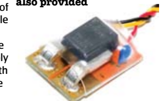
Above: Solder on your choice of connectors and put the current sensor in line to see what loads you draw
