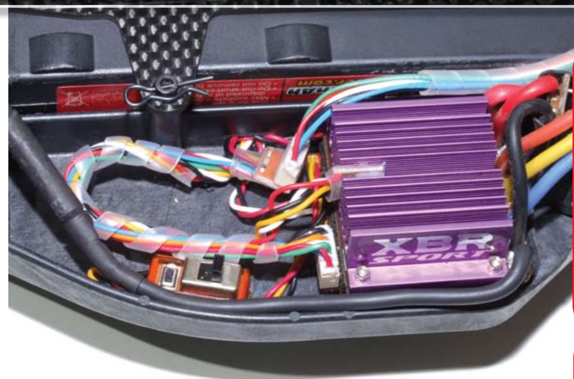
Above: The rpm sensor cable adapter installed, voltage cable and a temp sensor squeezed into the heatsink
