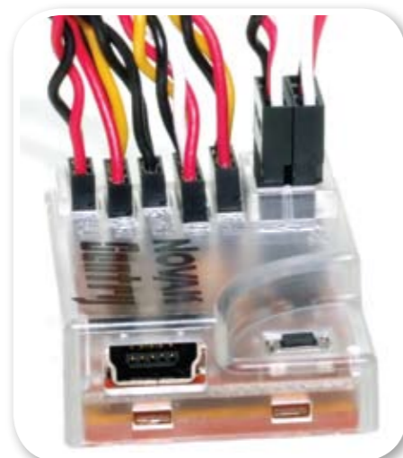
Above: The USB port connects direct to the PC, push button starts and stops recording
