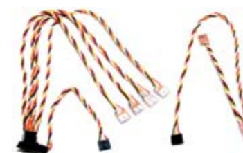
Above: The four additional digital temperature sensors have a port to accept the original two, making six in all! Below: The analogue temperature sensor is looped for fitting to nitro cylinder heads, motor end bells etc.
