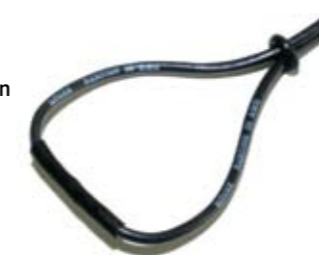
Above: The four additional digital temperature sensors have a port to accept the original two, making six in all! Below: The analogue temperature sensor is looped for fitting to nitro cylinder heads, motor end bells etc.
