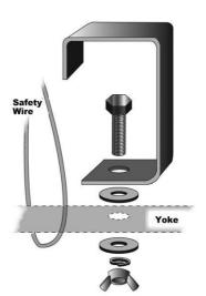
**NOTE**: Use washers and spring washers when attaching your hook clamp to the yoke.
