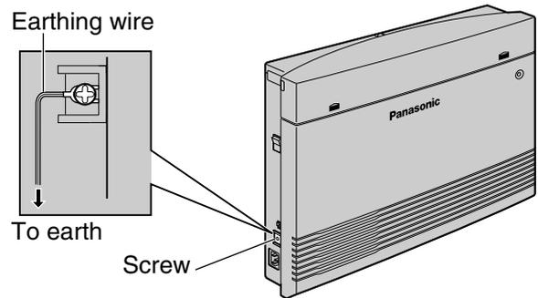
\* Use an earthing wire that has a conductor with a cross-sectional area of at least 0.75 mm<sup>2</sup> or 18 AWG. Green-and-yellow insulation is required.
