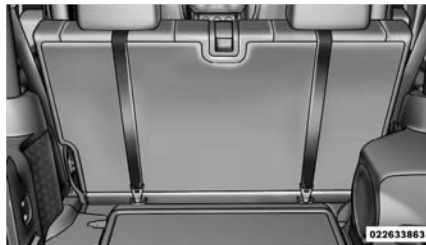
Tether Strap Mounting (Two-Door Models)
