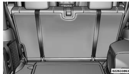
Tether Strap Mounting (Two-Door Models)
