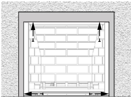
4. In the middle of the fireplace's black sheet metal front plinth, drill through the two dimples with an 1/8" bit.
