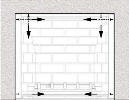
3. Install the backing plate with the four screws provided, fixing it at the top and on each side, as shown.
