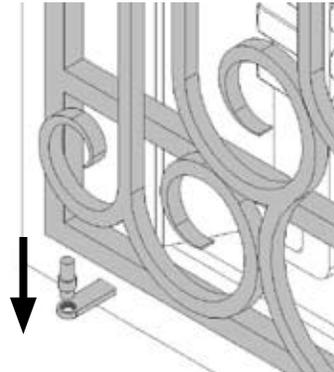
8. Align the top of the door under the upper hinge bracket. Drop the top hinge pin through the bracket, in the door frame. Repeat with the other door.
