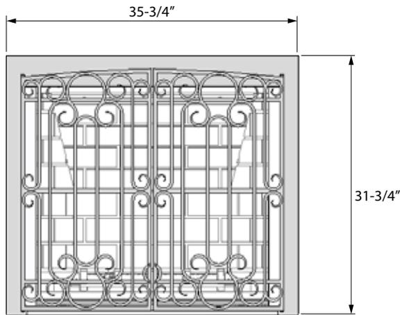
**NOTE:** The bottom of the plate is flush with the bottom of the heater. Bottom of the heater **MUST** be flush with or higher than the finished hearth.
