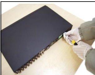
① disassemble the screw
