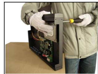
③ fix the screw of hard disk
