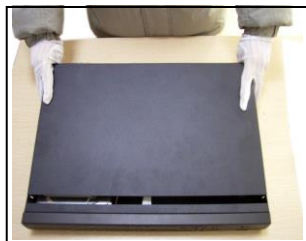
② disassemble the cover
