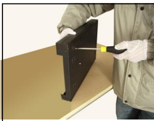
④ fix the screw of hard disk
