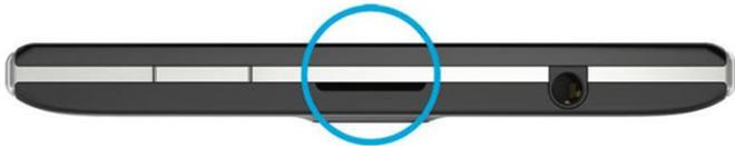
2. With the metal contacts facing away from you, insert the nano SIM card into the right slot.
