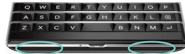
**NEW:** The BlackBerry Passport smartphone has an excellent speakerphone, providing clarity and volume in a small package. The phone uses a third-generation virtual back volume technology that makes audio louder and clearer without significantly increasing the physical size of the speaker box.
