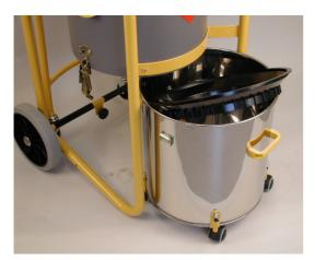
The collection container is fastened to the filter container with two large container clips. The wheels under the collection container make the emptying easier.
