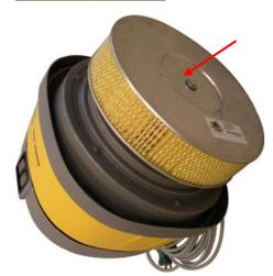
The motor top is provided with a HEPA-filter dust class "H". The filter holds back the finest and smallest dust particles that are not held back by the multi-tube filter. The filter holds back particles >0.3  $\mu m$  (0.0003 mm). The actual filter surface is 2.2 m² and is protected by a metal grating.
