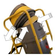
The very fine particles will be held back by the HEPA-filter under the motor top. The HEPA-filter will hold back the particles larger than 0.0003 mm.
