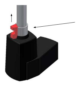
The lifting motor is equipped with a manual emergency lowering. In order to activate it, pull the red handle upwards.
