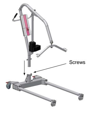
**Warning:** The top part must be mounted with the arm pointing forward, between the legs. Make sure not to mount the top part pointing the wrong way, as the lift will become unstable and unsuitable for lifting.
