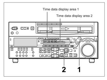
1 Press the RECORDER button or PLAYER button to select the VTR on which you wish to check the edit point.
