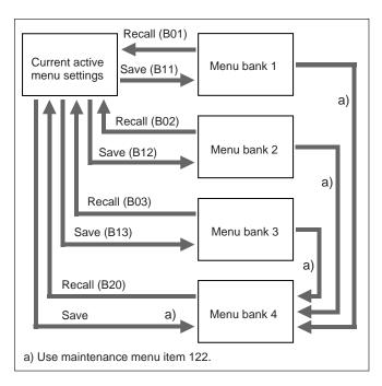
The current active setup menu settings as well as settings saved in menu banks are stored in separate storage areas for 525-line and 625-line modes.
