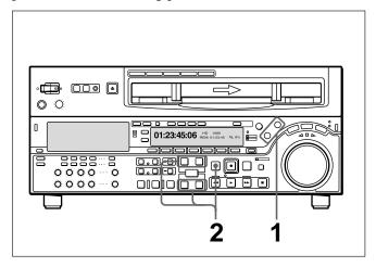
1 Press the RECORDER button or PLAYER button to select the VTR on which you wish to operate.
