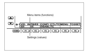
In the figure above, SDI (HD Serial Digital Interface signal) is selected as the setting for VID.IN (imput video signal selection), the menu item for button F1. This manual refers to this as "F1 (VID.IN) in function menu HOME page is set to SDI."
