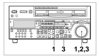
1 Press the SHUTTLE button or search dial so that the SHUTTLE button is lit.
