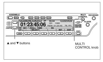
When the menu item number displayed in the menu display is flashing, you can change the menu item by turning the MULTI CONTROL knob.
