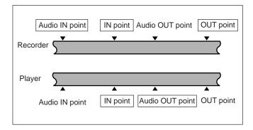
You can set audio cut in, crossfade, fade in, and fade out effects, including their durations, by menu selection. For details, refer to the Installation Manual.
