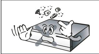
Keep the unit free of dust. Dust or metallic particles that find their way into the unit can cause fire or electric shock.
