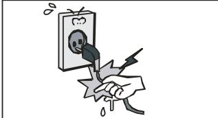
Do not unplug the unit by grabbing the cord. Turn off the power at the point, and firmly pull the plug. Do not move the unit while the power cord is plugged in.
