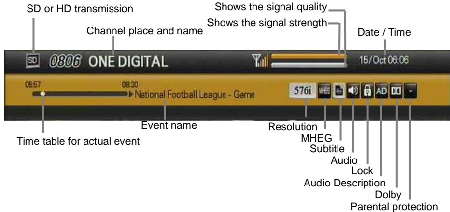
1. Press the **INFO** button to display the channel Information bar for a few seconds. The display duration is set in the OSD Display MENU.
