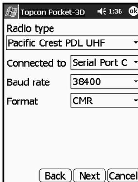
Figure 2-3. Radio Setup Dialog Box
