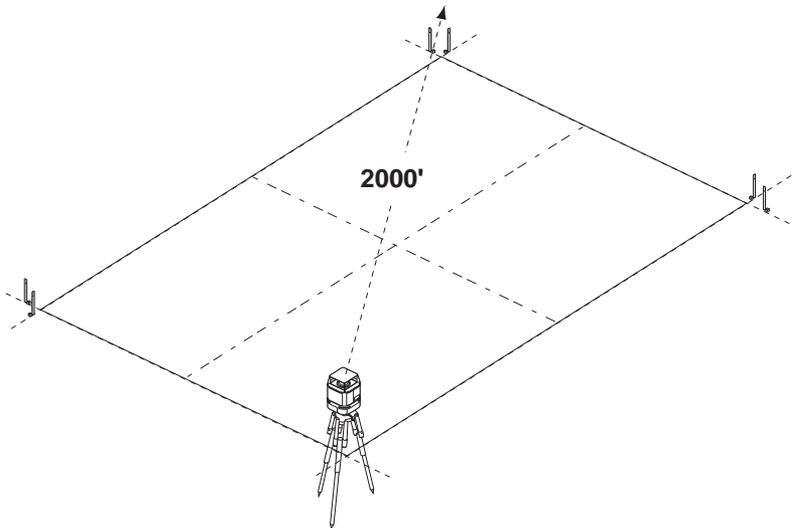
**Figure 1-15. Laser Transmitter Placement – Small Project**
