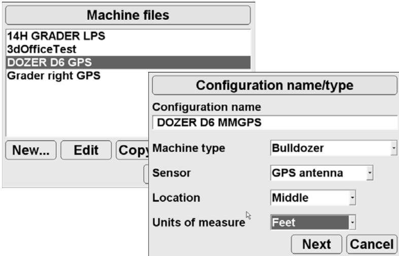
Figure 3-1. Enter Machine Configuration Information
