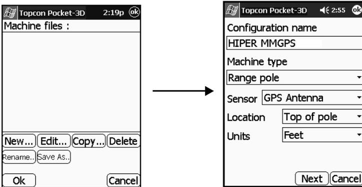
Figure 2-1. Create or Edit an Equipment Configuration
