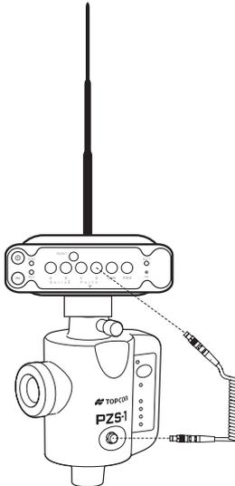
Figure 1-12. Receiver and PZS-1 on Rover Pole
