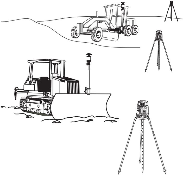
**Figure 1-17. Multiple Laser Transmitter Placement**
