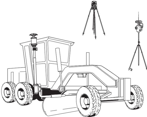
**Figure 1-1. System Five-3D with mmGPS**
