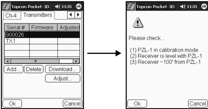
Figure 4-6. Begin Field Calibration Adjustment
