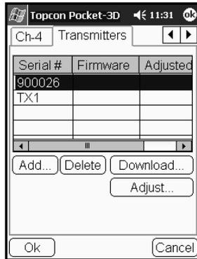
**Figure 2-8. Load Transmitters into Pocket-3D**
