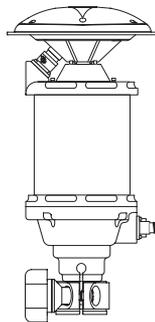
Figure 1-9. PZS-MC Machine Control mmGPS Sensor
