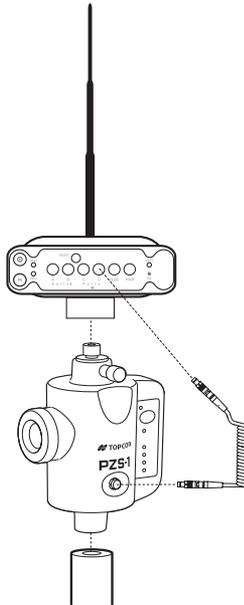
Figure 2-10. Connect Receiver and Sensor
