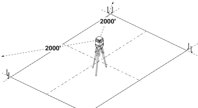
**Figure 1-16. Laser Transmitter Placement – Larger Project**
