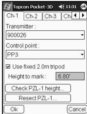
**Figure 2-9. Enter Transmitter Channel and Control Point Data**
