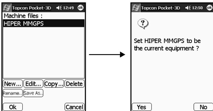
Figure 2-5. Select Equipment Configuration
