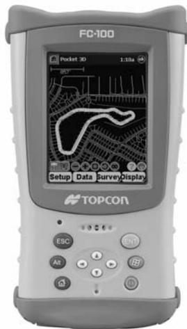
**Figure 1-13. Pocket-3D with mmGPS on the FC-100**
