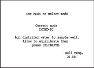
**G.** Apply enough distilled water to cover the the prism surface, allow to temperature equilibrate and press "**CALIBRATE**".
