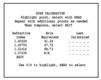
I. Adjust the refractive index value which should now be displayed, to the value listed on the bottle of calibration fluid by pressing "SET UP". Use the up/dwn/left/ right keys to adjust value. When the value matches press "READ" to accept and continue. Adjust temperature coefficient value or press "READ" to continue. Change reference temperature or press "READ" to continue. If the displayed value matches the value as listed on the bottle of calibration oil, press "CALIBRATE" to continue.
