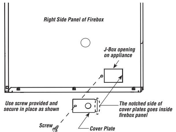
Figure 25 - Installing J-box Cover Plate - All Models
