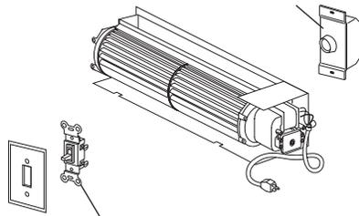
An ON/OFF wall switch can be used with the FBK-100 models (field supplied or order P/N 85L87 Wall Switch Kit, shown below)
