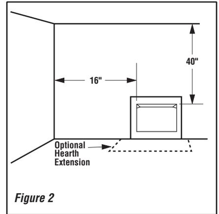
**Ceiling clearance:** The ceiling must be at least 40" from the top of the firebox opening (**Figure 2**).
