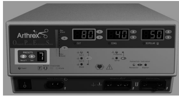
Figure 2 – 2 Controls for setting and recalling presets
