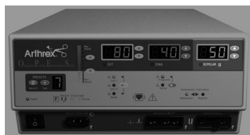
Figure 2 – 5 Controls for the Bipolar mode
