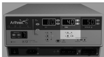
Figure 2 – 4 Controls for the Coag mode
