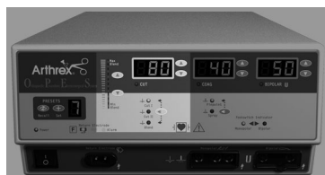
Figure 2 – 3 Controls for the Cut and Blend modes
