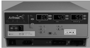
Figure 2 – 6 Indicators for power, return electrodes, and footswitch control
