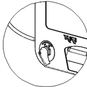
SWITCH ASSEMBLED TO BRACKET
