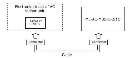
Do not modify the length of the cable supplied with the interface, it may affect to the correct operation of the interface.
