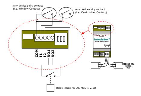
The relay output is also a dry contact normally open that can actuate any device with the following restrictions: 30VDC/5A, or 250VAC/5A max.
