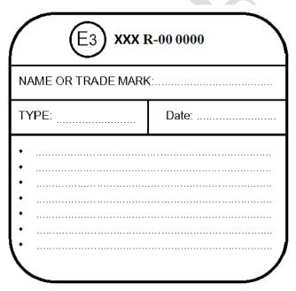
The above plate, with approval mark and some technical information on the HDDF retrofit system, has to be permanently fixed on the body of the vehicle.
