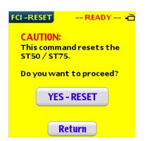
• Tap on the "YES – RESET" button. At this time the ST50/ST75 will break the communication link and the Configuration Software will respond with an error message. Communication has to be re-established with the ST50/ST75.
