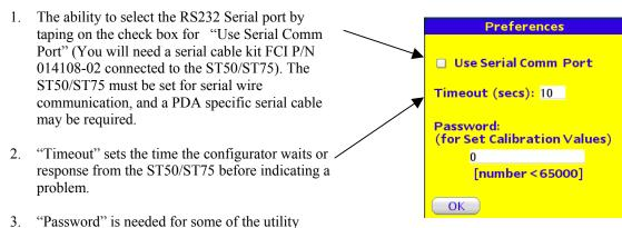
**NOTE:** When using the Configuration Software and the ST50/ST75 in serial cable mode, remember to change the jumper (JP5) in the ST50/ST75 to RS232 communication position.
