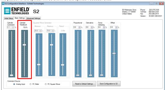
d. The position of the cylinder will be shown on the Cylinder Feedback slider
