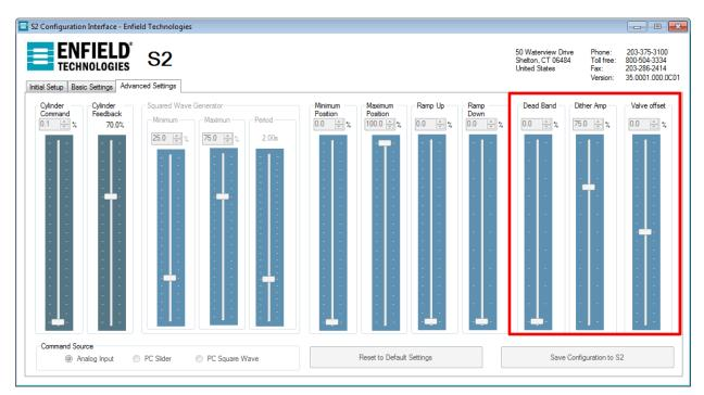
Dead Band – Adjusts the effective overlap of the valve. By increasing the Dead Band slider, the valve will begin to open sooner.
