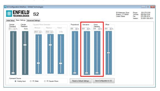
j. If an offset is noticed between the Cylinder Command and Cylinder Feedback sliders, the Offset slider can be adjusted to compensate. This is most likely the case in vertical applications. Assuming no mechanical linkages reversing direction of motion: for cylinder with rods facing up, increase the offset and for cylinders with rods facing down decrease the offset.
