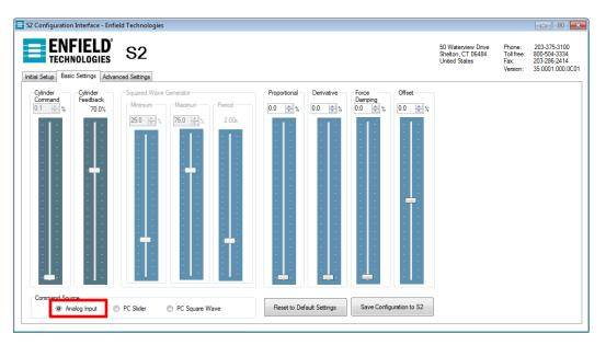
I. Confirm that the system is responding to your analog input signal. You will be able to see the Cylinder Command slider moving in unison with your command signal. If this does not happen, confirm your command source and wiring.
