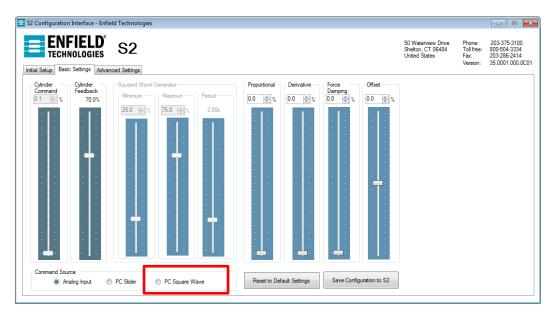
d. This will provide a text command signal that alternates between the two positions set by the Minimum and Maximum sliders, shown in the red box below. The Period slider will determine the amount of time for each cycle. To begin testing, use a signal such as 25% Minimum, 75% maximum and 4.00 Second for Period.
