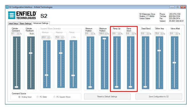
By increasing the ramp up, the velocity of the cylinder in the extend direction will be decreased. By increasing the ramp down, the velocity in the retract direction will be decreased
