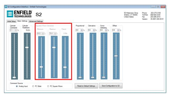
e. Increase the Proportional slider slowly (1% increments). The system should begin to move. If the system is not responding or is stuck in the fully extended or retracted position check tubing and feedback sensor polarity.
