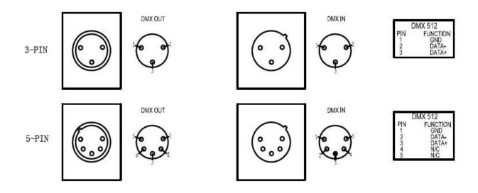
Connection between the controller and a projector and between one projector and another must be made with a 2 core-screened cable, with each core having at least a 0.5mm diameter. Connection to and from the projector is via cannon 3 pin (which are included with the projector) XLR plugs and sockets. The XLR's are connected as shown in the figure above.
