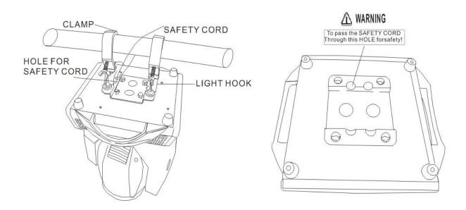
Use 2pcs clamp and 1safety cord(need to purchase). Use clamp fix with light hook which in the packing box with light, then use screw install to the bottom of lamp. Hang the fixture on the structure and fasten the screws attached to each clamp. Make sure the light is installed reliable, and confirm the light which you fixed is strong enough for hanging the light. Base on safety reason, please according to the above picture using safety wire cross the light to make it strong enough again.
