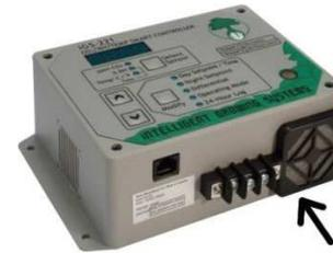
The controller is equipped with an internal fan that allows a faster air sampling. Do not expose the venting slits to potential sources of humidity or dust. These slits located under the control module are protected by a dust guard filter that should be there at all times. We recommend to regularly clean or replace the dust guard filter to improve the controller's effectiveness and its length of life.
