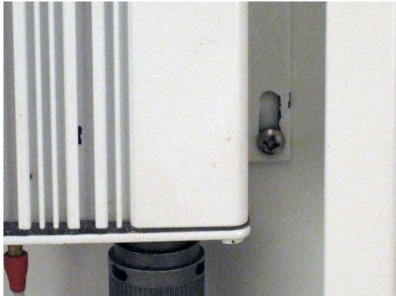
Figure 2. Proper mounting position of the electronics box.
