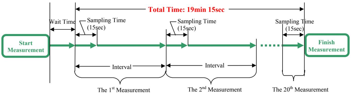
If the time period between two samplings is 10 seconds or longer, the pump will be turned OFF after a sampling is finished. Then the pump will be turned ON again 10 seconds before the next sampling starts.
