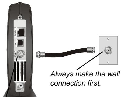
Before you connect or disconnect the USB or Ethernet cable, *always touch the coaxial cable connector on the cable modem.*
