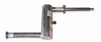
A Cryovent offers a reliable method to maintain liquid nitrogen or liquid argon in your vacuum insulated piping system. It requires no electricity to operate. A float operated valve allows gas to be vented from the system to ensure a liquid full piping system.
