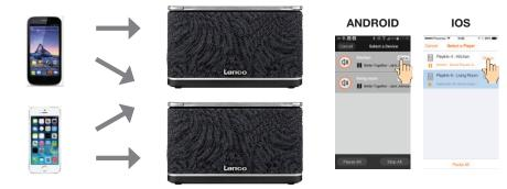
If several speakers are connected simultaneously on your home network, you can play indifferently a song on speaker 1 and another song on the speaker 2 from any mobile device connected to the network.
