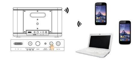
The LED indicator is flashing a few times, after which it becomes permanent white: the speaker becomes detectable as a WiFi access point.
