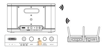
Press the WPS key of the router and the Quick Connect key of the speaker simultaneously. The LED on speaker is flashing fast (white). After around 10~40 seconds, the Wi-Fi LED on speaker becomes stable white: The speaker is connected to your network.
