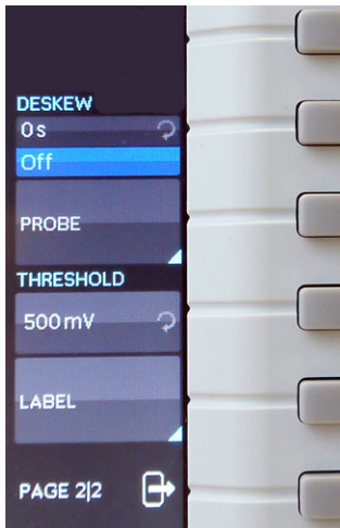
Fig. 2.6: Basic soft menu elements for settings and navigation
