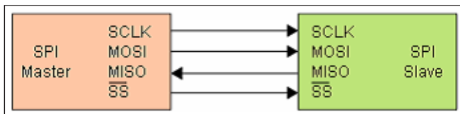
Fig. 12.9: Simple configuration of a SPI BUS
