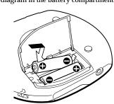
To remove the batteries Remove the batteries as illustrated below.
