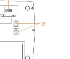
24 Fuses25 Battery Compartment26 Wall-mounting Holes
