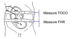
Figure 8-1 Positioning transducers (single fetus)
