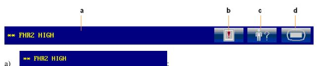
Alarm messages displaying area. When an alarm is active, the message will be displayed here in yellow. Patient alarms will be displayed on the left and technical alarms in the center.
