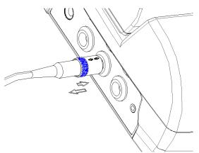
When disconnecting a transducer, hold the afterbody of the transducer outshell (the shaded part shown in figure 6-2) with fingers and push it in slightly, then pull it out. Refer to figure 6-2.
