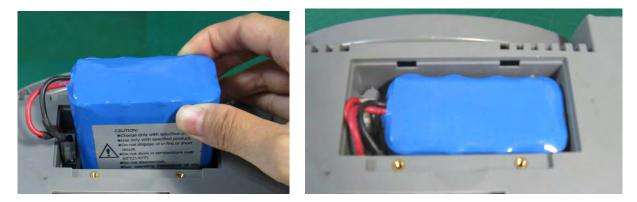
6) Shut the battery compartment cover and fix the screws.
