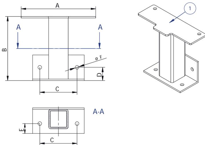
1) Mounting surface to be attached to burner
