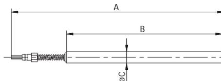
**Spark ignitor - quartz with tube**
