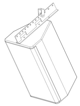
Using the supplied M10 hex head bolts, align the mounting holes in the flying bracket with the mounting points on the top or the bottom of the enclosure. Ensure that both the flat and locking washers are used — the flat washer should be in contact with the cradle. Tighten the bolts to ensure a solid fit. Finally, attach a hook-clamp to the mounting point and secure the mounting point bolt through the main section of the flying bracket.
