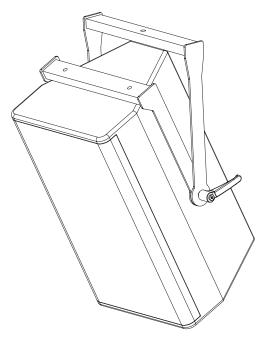
Attach the coffin plate to the inner yoke using the supplier M8 countersunk bolts, flat washers and Nyloc nuts. Ensure the washers are placed between the yoke and the locking nut.
