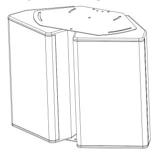
Using the supplied M10 socket head bolts, bolt through the CP-XY12DF1 plate into the enclosures. Ensure that both the flat and spring washers are used — the flat washer should be in contact with the plate. Once the desired angles of the loud-speakers are set, tighten the bolts to lock in place. Then turn the cluster over and repeat the process on the bottom. Use the rear points on the XY-122 enclosures, or the M10 holes on the CP-XY12DF1 plates to use as a secondary safety feature.
