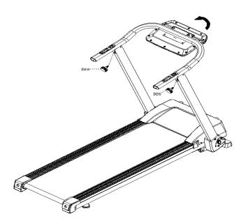
Step 4: Put on the SAFETY KEY (14) and Mp3 line(C25)
