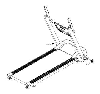
**STEP4**: according to the picture to tight the M12 Knob(D25)
