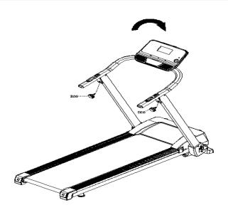
**STEP 3**:according to the picture to loose the M12 Knob(D25)
