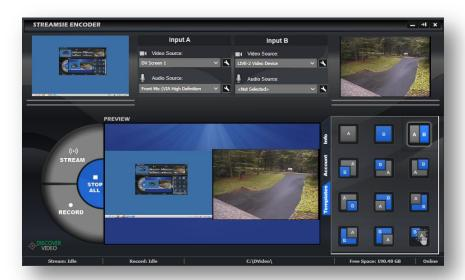
Streamsie PC supports one or two video inputs which may be selected from the Video and Audio Source dropdown selectors. For example, Input A might be camera 1 and Input B might be camera two. Or Input A might be your computer screen and Input B might be a camera. Similarly, select the desired audio inputs.
