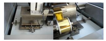
Normally loosen the housing screw first then turning the adjusting screw, last tighten the housing screw after adjusting right.
