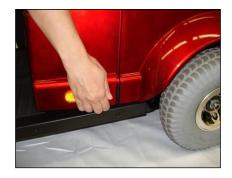
Remove the battery cover by loosening the elastic belt on the front of the cover and the Velcro on either side of the battery cover.
