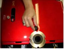
Loosen the rear cover from the rear frame by turning the rotary knob in an anticlockwise direction and by loosening the Velcro on both sides inside the cover.
