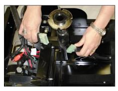
Disconnect the main cable before dismantling the scooter's frame components.
