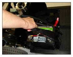
Remove the batteries by lifting them up using the straps.
