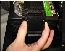
Undo the belt holding the battery in its place.
