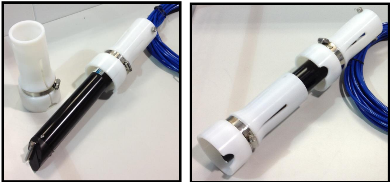
Figure 1-4: ABS Deployment Guide installed on a DTS-12
