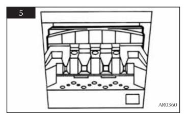
6.3 Locate the front coal between the heat shield and flame baffle so that its ends sit flat against the burner skin, see diagram 6.
