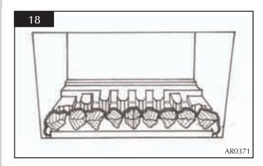
5.16 Place three large coals on the front coal so that they lean against the flame baffle and four large coals on the flame baffle so that they sit on the fingers, see diagram 19.
