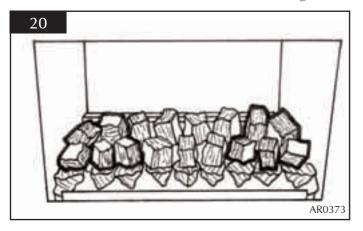
518 Place six small coals along the rear of the flame baffle, resting against the rear ledge, see diagram 21.
