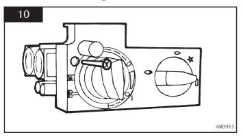
6.4 To release the right-hand side of the control cover, insert the narrow blade screwdriver into the slot shown in diagram 11. Lever it gently and pull from the right-hand side at the same time. The cover will now come off. There is a small cylindrical metal spacer inside the cover. This must be kept and replaced on the fixing screw during re-assembly.
