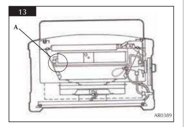
8.2 Rotate the injector until it is fully removed, and install the correct replacement injector. Reassemble and turn the gas supply on, check for leaks.
