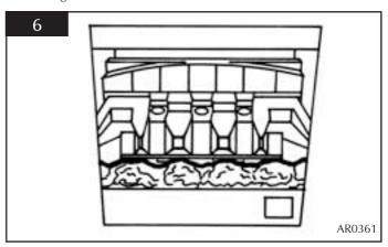
5.4 Place five of the loose round coals on the front coal so that they lean against the flame baffle, in between the fingers. Place the two rectangular coals behind the round coals, one at each side, see diagram 7.
