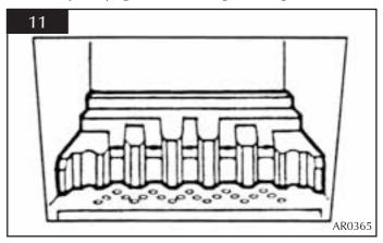
5.9 Locate the front coal moulding in front of the flame baffle ensuring that the end legs sit flat against the burner skin, see diagram 12.
