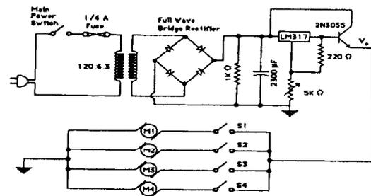
Electrical circuitry. M1, M2, M3, and M4 are the four vibrators.
