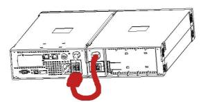
1500/2000VA model only: connect the UPS power cord to the mains power supply.
