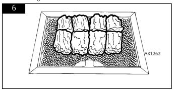
5.4.2 Place 14 small coals or pebbles around the edge of the tray as shown, ensure that there are gaps between each coal or pebble. Place one on top of the pilot shield. See diagram 7.
