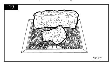
7.7.4 Place log (No. 7) along the LH side of the tray, log (No. 9) along the RH side of the tray and place logs (No. 8 and 11) along the front of the tray as shown. Place the cone (No. 14) on the LH side of the burnt log. See diagram 20.
