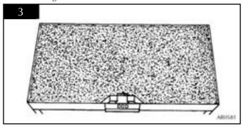
7.3.4 Smooth out the fire beads, it is important to ensure that the fire is completely filled, level to the top.
