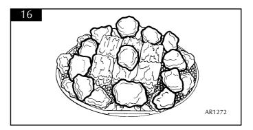
5.6.4 Place the remaining 4 large coals or pebbles on top of the square blocks, ensure that they lean against the central small coal or pebble and that there are gaps between each coal or pebble. See diagram 17.
