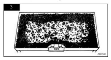
5.3.3 Using the small beads, fill the fire to the top. See diagram 4.
