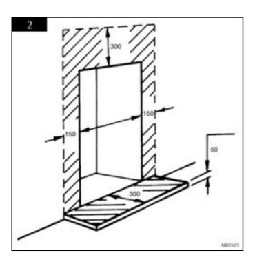
4.8 The following table indicates the minimum opening sizes for each model. In each case, a gap of 20mm has been allowed to both Left and Right of the basket. See diagram 3.
