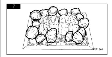
7.4.4 Place the remaining 6 large coals or pebbles on top of the square blocks, ensure that there are gaps between each coal or pebble. See diagram 8.
