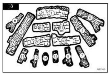
5.7.2 Place the two logs (No.13) on top of the beads as shown. See diagram 19.
