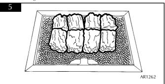
7.4.2 Place 14 small coals or pebbles around the edge of the tray as shown, ensure that there are gaps between each coal or pebble. Place one on top of the pilot shield. See diagram 6.
