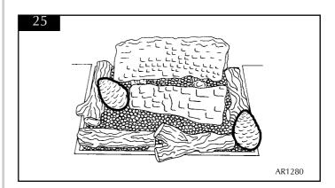
7.8.5 Place one large log (No. 6) so that it rests on top of the rear and front logs to the LH side. Place the other large log (No. 6) so that it rests on top of the rear and front logs on the RH side and log (No. 8) so that it bridges the centre gap as shown. See diagram 26.
