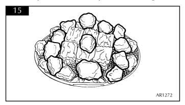
7.6.4 Place the remaining 4 large coals or pebbles on top of the square blocks, ensure that they lean against the central small coal or pebble and that there are gaps between each coal or pebble. See diagram 16.
