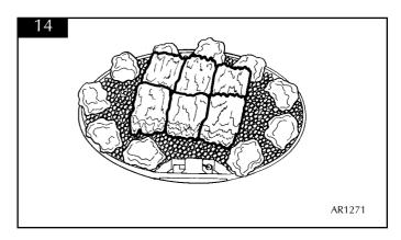
7.6.3 Place one large coal or pebble on top of the pilot shield, then place 10 alternating large and small coals or pebbles around the perimeter of the fire. They should sit on the bottom row of small coals or pebbles and rest against the inner mass of square blocks. Place one small coal or pebble on top of the centre of the square blocks. See diagram 15.
