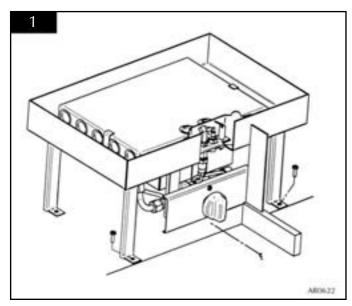
1.5 Lift the fire away from the hearth and carefully tip the firebeads (or glass granules if applicable) into a dry clean container for later replacement.
