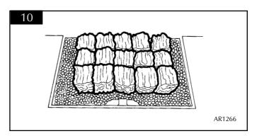
5.5.2 Place 18 small coals or pebbles around the edge of the tray as shown, ensure that there are gaps between each coal or pebble. Place one on top of the pilot shield. See diagram
