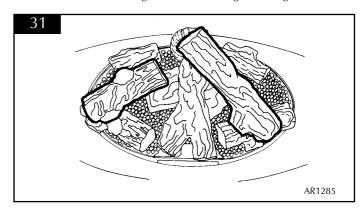
7.9.6 Place the two thin logs (No. 12), one at each side sitting on the tray and resting against the previously positioned logs.Place one log (No. 9) at the LH rear resting on the base log, and one log (No. 8) at the RH rear. See diagram 32.
