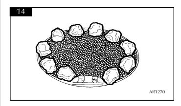
5.6.2 Place 6 large square blocks in a solid mass in the centre of the burner tray as shown, ensure they fit tightly together. See diagram 15.
