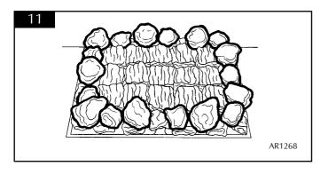
7.5.4 Place the remaining 11 large coals or pebbles on top of the square blocks, ensure that there are gaps between each coal or pebble. See diagram 12.
