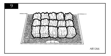
7.5.2 Place 18 small coals or pebbles around the edge of the tray as shown, ensure that there are gaps between each coal or pebble. Place one on top of the pilot shield. See diagram 10.
