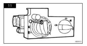
8.4 To release the right hand side of the control cover, insert a narrow blade screwdriver into the slot shown in diagram 12, lever it gently and pull from the right hand side at the same time. The cover will now come off. There is a small cylindrical metal spacer inside the cover, this must be kept and replaced on the fixing screw during re-assembly.
