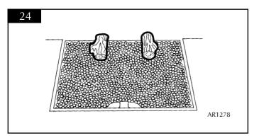
5.8.3 Place the large log (No. 1) so that it sits on top of the previous two logs. Place the burnt effect log (No. A1) in the centre of the tray as shown. Place one log (No. 7) along each side of the tray, another log (No. 7) along the front LH side and a log (No. 8) along the front RH side of the tray. See diagram 25.
