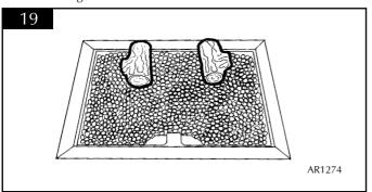
5.7.3 Place the large log (No. 1) so that it sits on top of the previous two logs. Place the burnt effect log (No. B1) in the centre of the tray as shown. See diagram 20.
