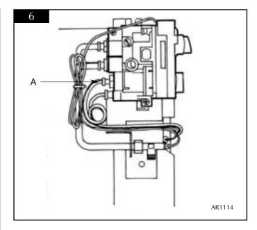
4.4 Undo the pilot pipe connection from the pilot unit, remove the 2 screws securing the pilot and remove the pilot assembly. See diagram 7.
