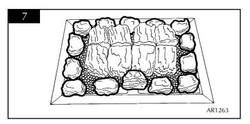
5.4.3 Starting at the front, place 14 alternating large and small coals or pebbles around the perimeter of the fire, they should sit on the bottom row of small coals or pebbles and rest against the inner mass of square blocks. See diagram 8.
