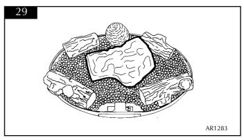
7.9.4 Place one log (No. 8) in the centre so that it rests on the rear cone and the pilot shield. See diagram 30.
