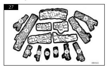
7.9.2 Place a cone (No. 14) in the centre at the rear edge of the tray and place one log (No. 13) at each side of the cone. Place one log (No. 11) along the front of the tray at each side of the pilot. See diagram 28.
