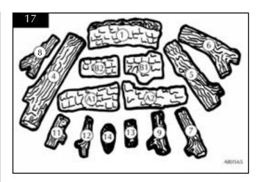
7.7.2 Place the two logs (No.13) on top of the beads as shown. See diagram 18.
