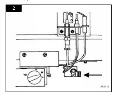
If the isolation tap is to be fitted under the fire, the GAZCO GC00060 provides a neat and easy solution.
