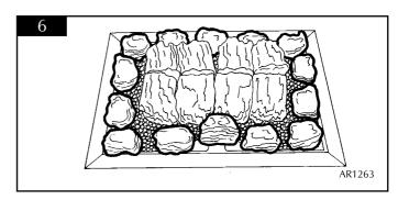
7.4.3 Starting at the front, place 14 alternating large and small coals or pebbles around the perimeter of the fire, they should sit on the bottom row of small coals or pebbles and rest against the inner mass of square blocks. See diagram 7.
