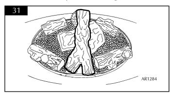
5.9.5 Place one log (No. 11) so that it rests on the LH front log and the burnt log. Place another log (No. 7) so that it rests on the RH front log and the burnt log. See diagram 32.
