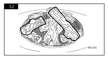
5.9.6 Place the two thin logs (No. 12), one at each side sitting on the tray and resting against the previously positioned logs. Place one log (No. 9) at the LH rear resting on the base log, and one log (No. 8) at the RH rear. See diagram 32.
