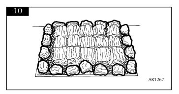
7.5.3 Starting at the front, place 18 alternating large and small coals or pebbles around the perimeter of the fire, they should sit on the bottom row of small coals or pebbles and rest against the inner mass of square blocks. See diagram
