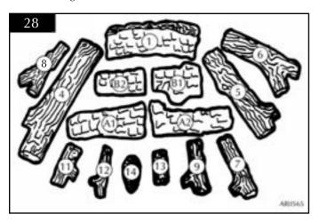
5.9.2 Place a cone (No. 14) in the centre at the rear edge of the tray and place one log (No. 13) at each side of the cone. Place one log (No. 11) along the front of the tray at each side of the pilot. See diagram 29.
