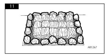
5.5.3 Starting at the front, place 18 alternating large and small coals or pebbles around the perimeter of the fire, they should sit on the bottom row of small coals or pebbles and rest against the inner mass of square blocks. See diagram 12.
