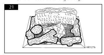
5.7.5 Place the large log (No. 6) so that it rests on top of the rear and front logs to the LH side, Place log (No. 7) on the RH side and log (No. 8) so that it bridges the centre gap as shown. See diagram 22.
