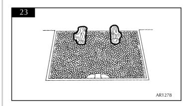
7.8.3 Place the large log (No. 1) so that it sits on top of the previous two logs. Place the burnt effect log (No. A1) in the centre of the tray as shown. Place one log (No. 7) along each side of the tray, another log (No. 7) along the front LH side and a log (No. 8) along the front RH side of the tray. See diagram 24.
