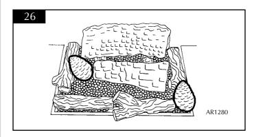
5.8.5 Place one large log (No. 6) so that it rests on top of the rear and front logs to the LH side. Place the other large log (No. 6) so that it rests on top of the rear and front logs on the RH side and log (No. 8) so that it bridges the centre gap as shown. See diagram 27.
