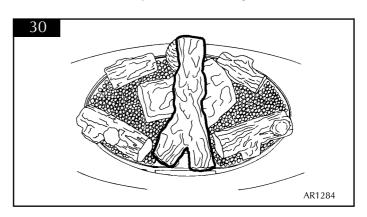
7.9.5 Place one log (No. 11) so that it rests on the LH front log and the burnt log. Place another log (No. 7) so that it rests on the RH front log and the burnt log. See diagram 31.
