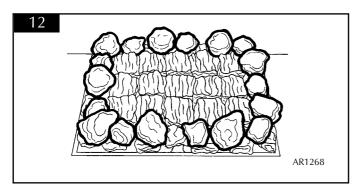
5.5.4 Place the remaining 11 large coals or pebbles on top of the square blocks, ensure that there are gaps between each coal or pebble. See diagram 13.
