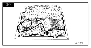
7.7.5 Place the large log (No. 6) so that it rests on top of the rear and front logs to the LH side, Place log (No. 7) on the RH side and log (No. 8) so that it bridges the centre gap as shown. See diagram 21.
