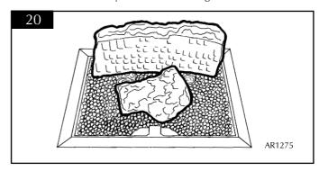
5.7.4 Place log (No. 7) along the LH side of the tray, log (No. 9) along the RH side of the tray and place logs (No. 8 and 11) along the front of the tray as shown. Place the cone (No. 14) on the LH side of the burnt log. See diagram 21.
