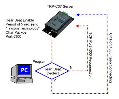
Step1: Run TRP-C37X DSM.exe to set up the heart beat enable.
