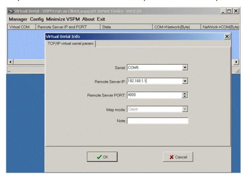
**Step8.** If Virtual-Com setting success, the display will appear bellow. **Step9.** Run TRPCOM utility then select virtual-com port make a TRP-C37 loop test.
