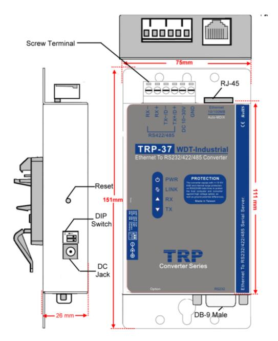
**Notice:** User can only choose either external DC-Jack or Screw terminal DC input. Do not use external DC-Jack and screw terminal DC input simultaneously.
