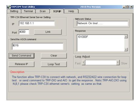
Step3.Send Command "#010003", The Response will enable TRP-C28 Relay1 and Relay2 enable.
