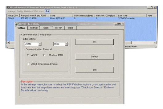
Step3.Select "Terminal" and send command, the response will appear TRP-C28 channel 2 counter value.
