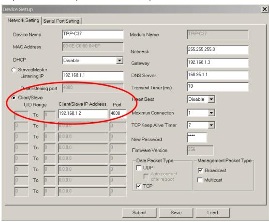
Step3.Run DSM set up *TRP-C37 Server* and be sure the IP and port as same as client setting. \*Adjust Maximum Connection to 16.
