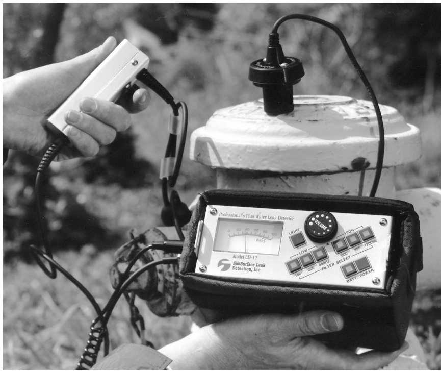
Figure 4-6 Leak Survey at a Hydrant
