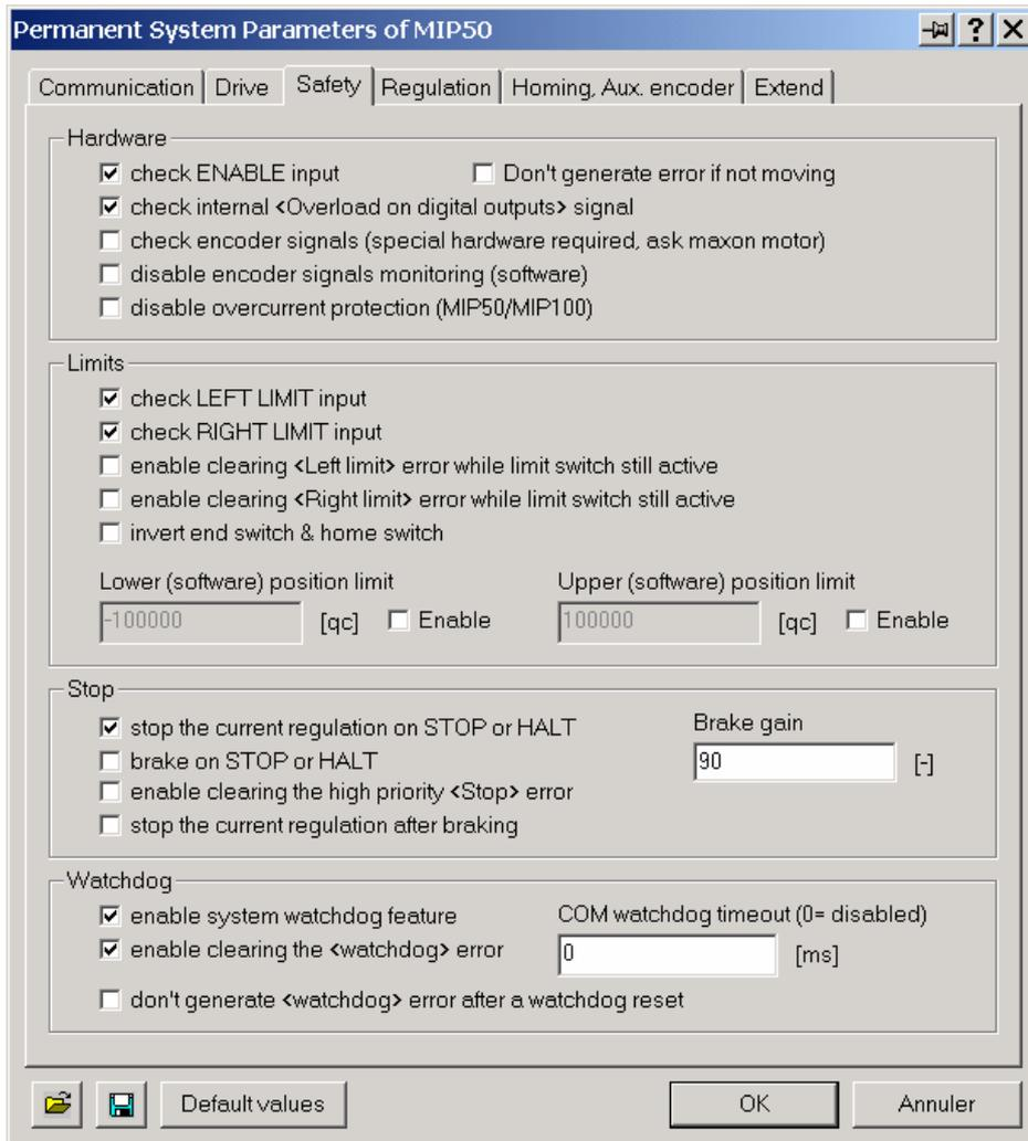
The default parameters offer a standard safety. Carefully read the information displayed in the yellow help window in order to optimize the safety for your particular drive system.
