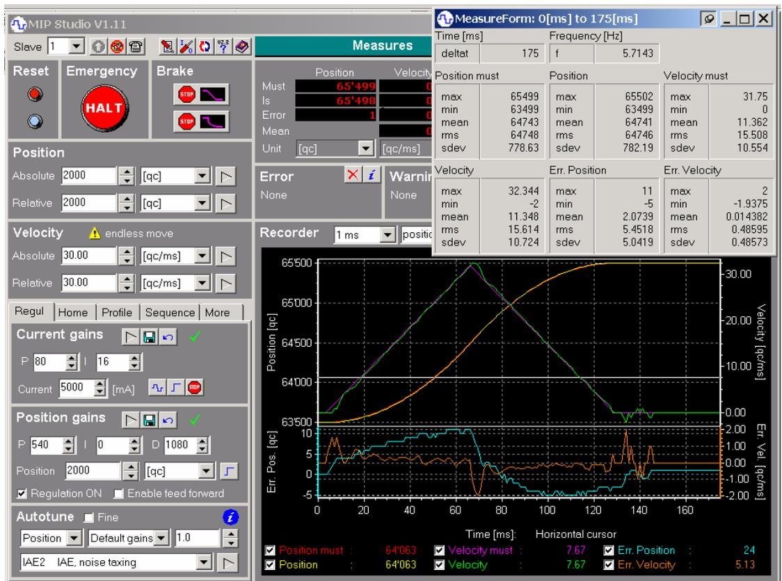
You can see the result in the 'Recorder' panel and judge the performance of the regulation. By pressing the 'M' key you will see statistical values (like the rms value of the position error) that will help for an objective performance analysis.
