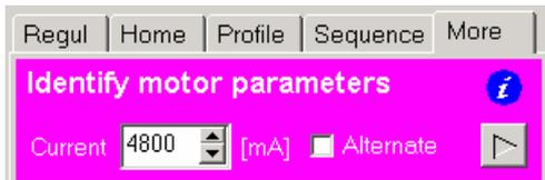
The 'Current' edit box limits the current that is used to identify the motor. Typically this current should be twice the nominal continuous current of the motor and less or equal to the peak current.
