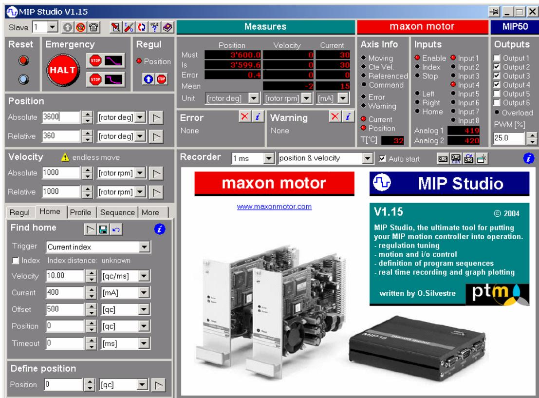
Before you can work with MIP Studio you will need to establish the communication with the MIP controller. In most cases the MIP controller and MIP Studio will not communicate in a first time, because the default factory settings for the communication are not compatible with MIP Studio (for compatibility with past firmware versions the factory settings are for 'Text menu' mode at 19'200 baud).
