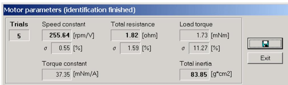
Normally the identified motor parameters should be preferred to the catalogue values since they incorporate the real measurement gain factor of the controller as well as the electrical resistance of the cabling and the real supply voltage.
