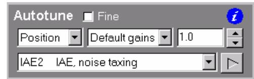
This will take a few minutes while you can follow the evolution of the gains and the cost function in the recorder area. At the end, the results are shown in a window. If the improvement factor is > 1.0 then the optimized gains are automatically saved to the system parameters.
