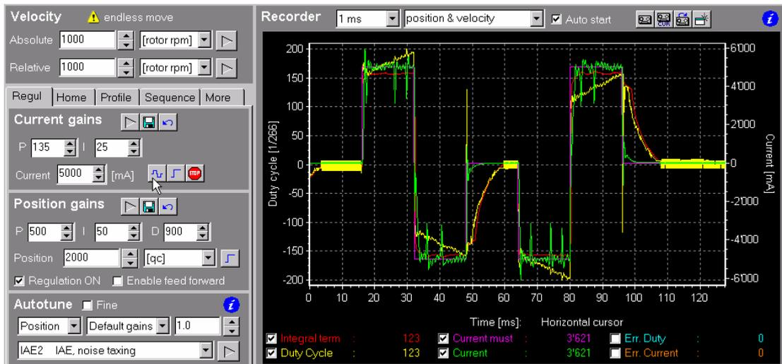
With EC motors you will notice short breaks in the current that correspond to the phase commutations (this is absolutely normal). The faster the rotor turns, the more phase commutations you have. On the MIP50 a flat integral term is a sign that the speed constant is correctly set in the system parameters.
